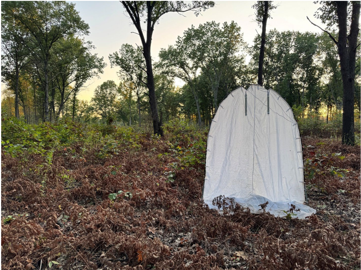
Ultraviolet blacklight station used to survey for rare moths in Metroparks Toledo. Photo from Dunes Trail on 09/25/2025.
