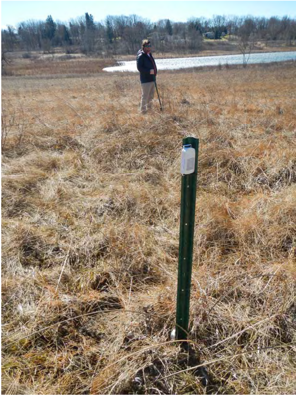
Figure 2. Photo of data logger placement (ground level and 1 meter elevated) at Eaton Road, Long Lake Fen, March of 2017 (Mike Losey, Springfield Township in background).
