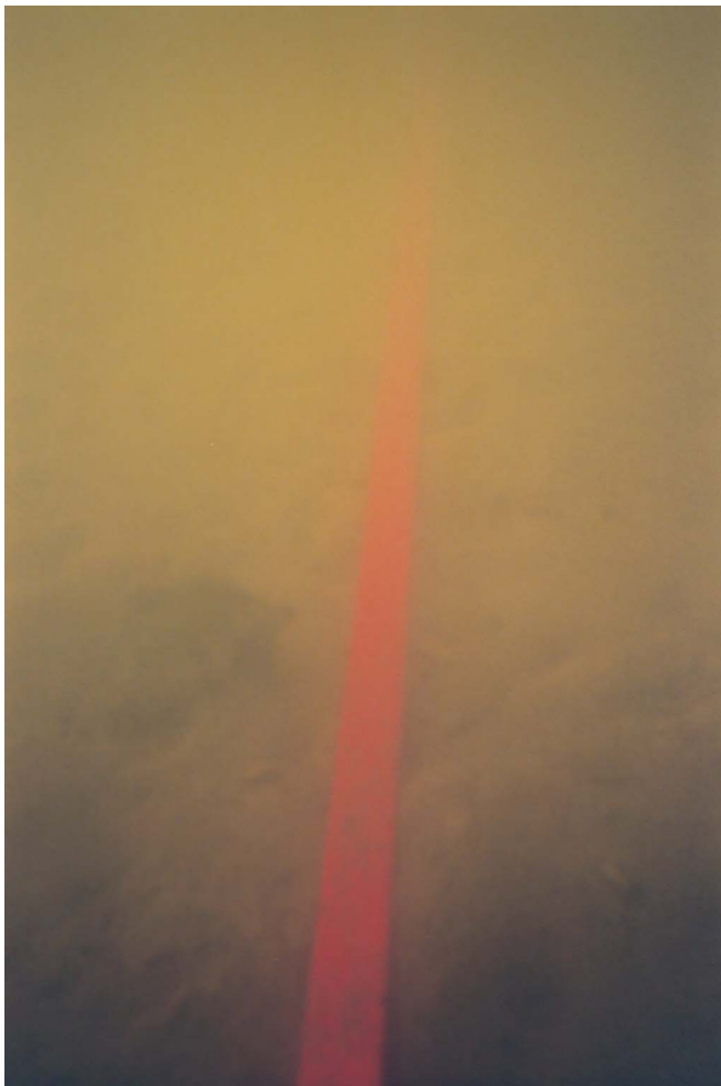
Figure 8. Transect line anchored to the stream bottom and ready for survey.
