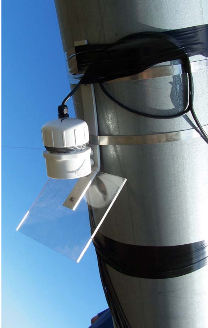
Figure 3. Two bathats were installed to house Anabat microphones and to collect bat acoustic data at 5 m and 55 m AGL in the Blissfield Wind Energy Project Area in Lenawee County of southeastern Michigan.
