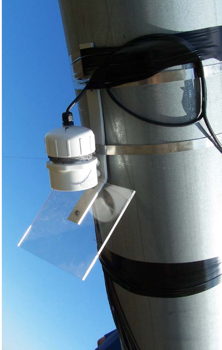
Figure 3. Two bathats were installed to house Anabat microphones and to collect bat acoustic data at 5 m and 75 m AGL in the Green River Wind Energy Project Area in Illinois.
