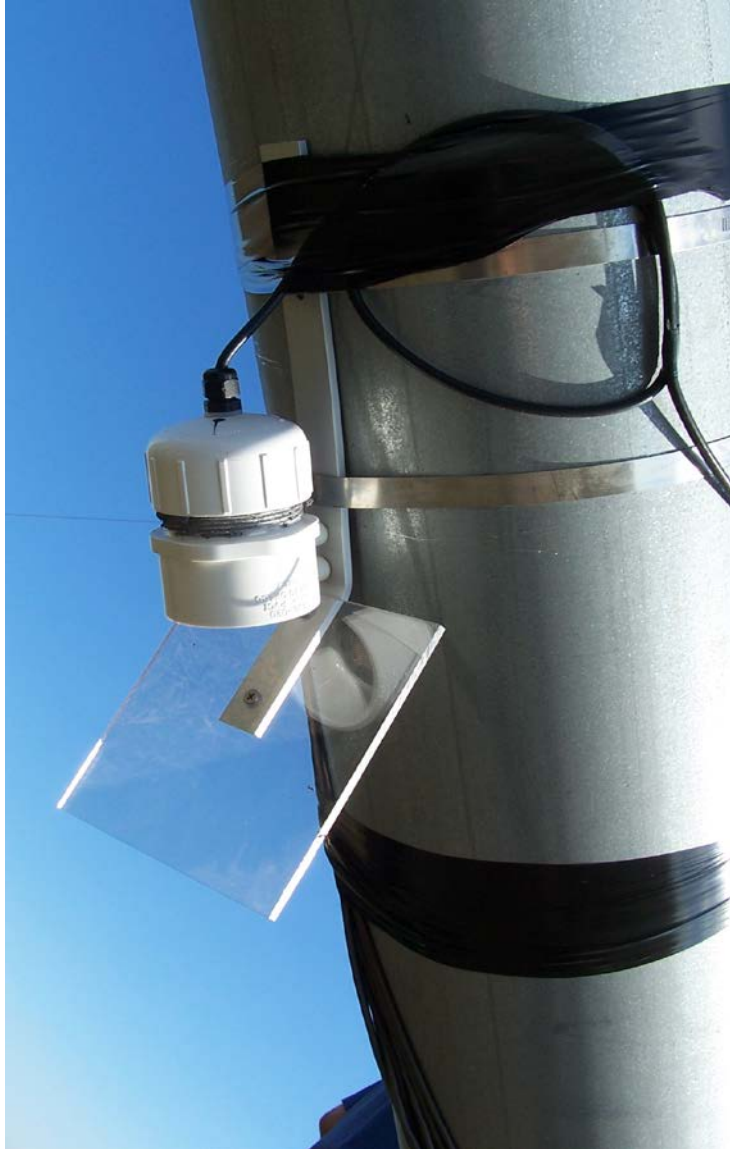
Figure 3. Two bathats were installed to house Anabat microphones and to collect bat acoustic data at 5 m and 55 m AGL in the Blissfield Project Area in Lenawee County of southeastern Michigan.
