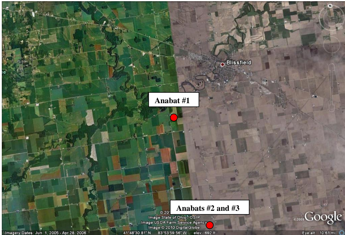
Figure 2. Three Anabats were installed to collect bat acoustic data in the Blissfield Project Area in Lenawee County of southeastern Michigan. Anabat #1 was located on the ground level, Anabat #2 was attached to a meteorological monitoring tower at 5 m above ground level, and Anabat #3 was attached to a meteorological monitoring tower at 55 m above ground level,
